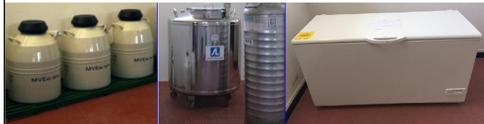
Below the text, there are three photographs of laboratory equipment: three white cylindrical liquid nitrogen tanks labeled 'MVE 300', two large stainless steel tanks on wheels, and a white horizontal deep freezer.
